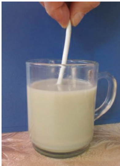
stirring of zeolite powder to a suspension with a ceramic spoon
